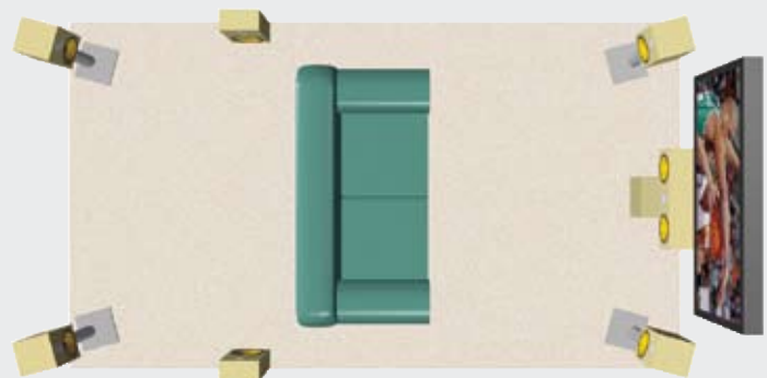
4-7: A "6.1/7.1" system adds speakers at the rear of your home theater room to reproduce "Center Surround" information contained in whatever source you are playing.
