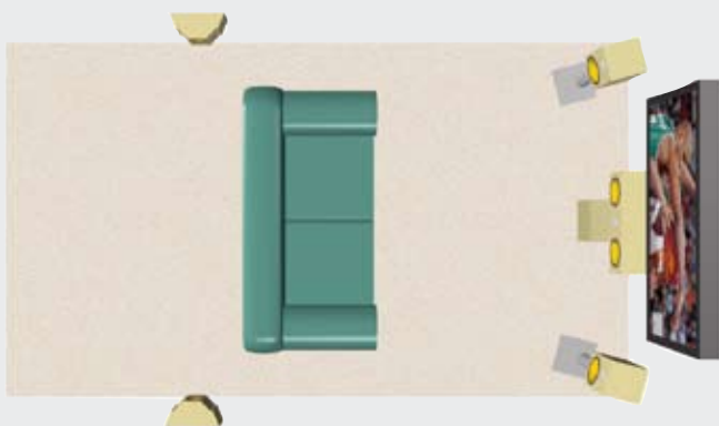
4-6: Dipole speakers create a very spacious but non-specific feeling of ambience.
