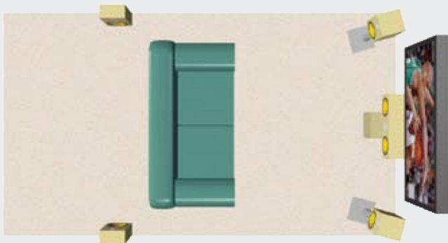
4-4: If you'll be listening primarily to movie soundtracks, place your surround speakers on the side walls just behind your main listening/viewing position.
